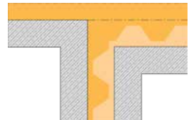
With temporary steel sheet pile retaining walls, the reinforced concrete structure built inside the excavation pit reduces the available surface
