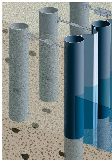
Tubular combined wall as retaining wall
