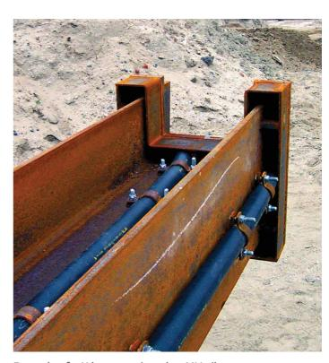
Example of a H beam equipped as MV pile
