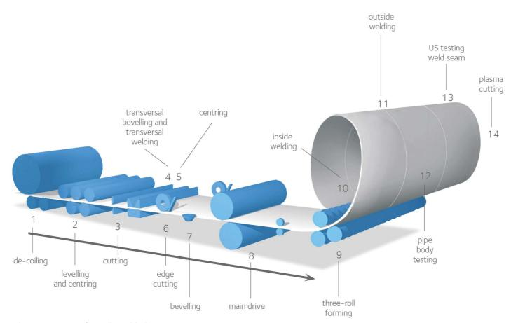
Production process of spirally welded pipes
