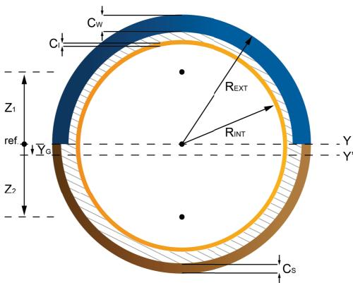
Figure: Tube surface with reduced area profile
