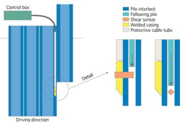
Schematic view of operating principle
