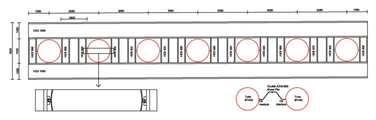
Two main types of driving templates exist: Single and double level. The most common is the single level template, however in certain cases a double level template can be used to ensure that the tubes are installed within the vertical tolerances. For driving tubes from water a floating or non-floating template can be used. Foundation Solutions has the capability to design and produce project specific driving templates on demand of the customer.
