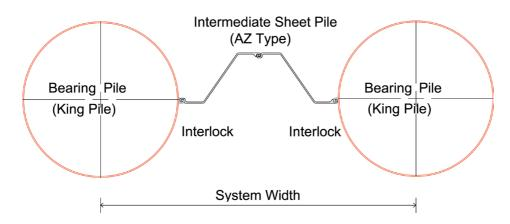
Tubular combined wall system with the different elements
