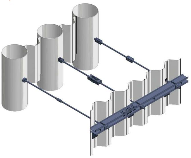
Anchoring a tubular combined wall using a tie back system can be quite simple and efficient. A tie rod links each tube to an anchor wall, which can consist of a sheet pile wall, steel tubes or even another combined wall.
