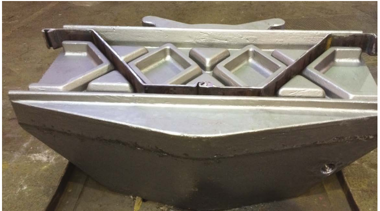
Cast steel driving cap
