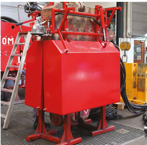
Sound insulation measures for hammer (up) and vibration bear (down)
