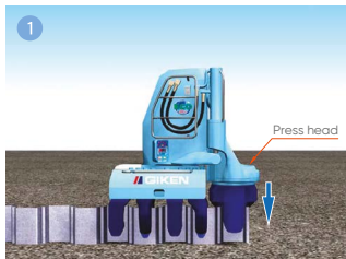
The sheet pile is completely pressed in.
