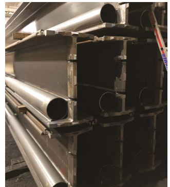
Factory-mounted inclinometer pipes; HZ ® -M beams with toe reinforcements and inclinometer pipes
