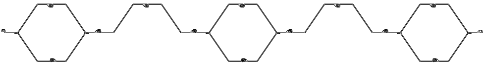
Z-box pile wall (CAZ): Design possible with intermediary piles or as a pure box pile wall
