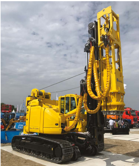
Two-way unit with short mast for pile driving along railway lines with limited working space to sideways and upwards.
