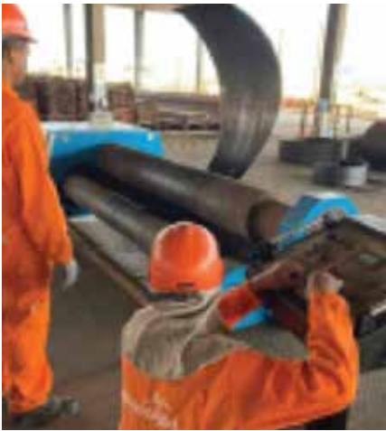
The plate is rolled into pipe
