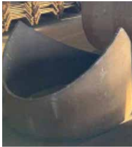
The pipe is cut into the required shape
