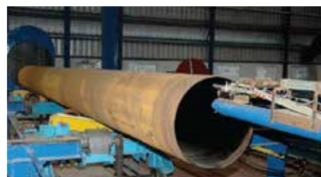
Internal Painting Line
