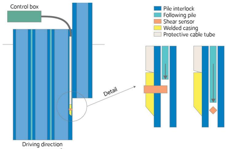
Schematic view of operating principle
