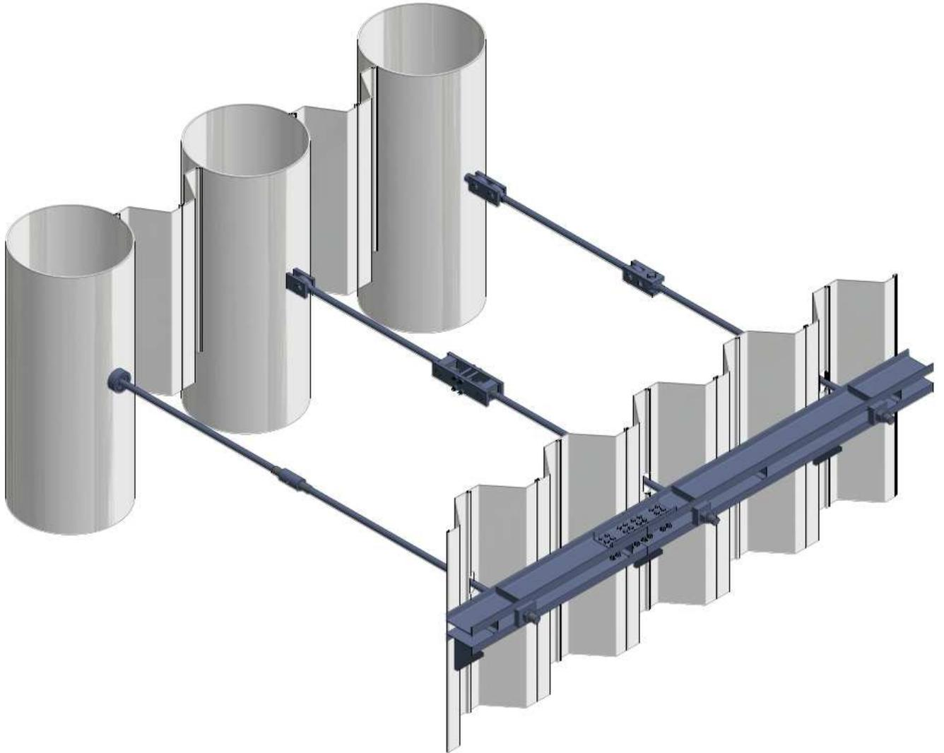
Anchoring a tubular combined wall using a tie back system can be quite simple and efficient. A tie rod links each tube to an anchor wall, which can consist of a sheet pile wall, steel tubes or even another combined wall.
