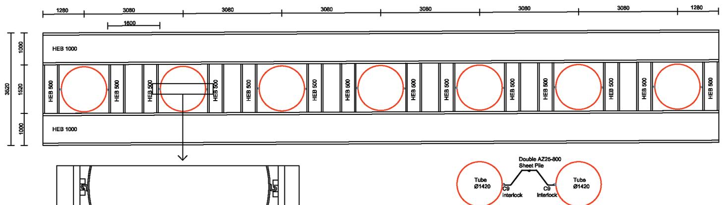
Schematic drawing driving template
