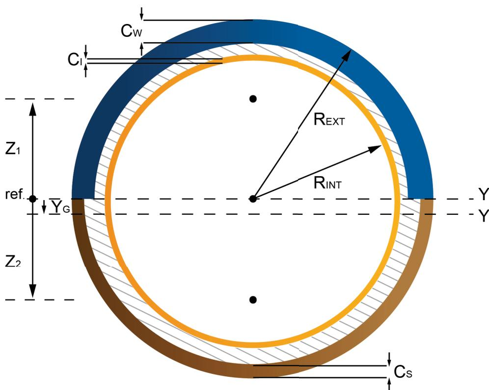
Figure: Tube surface with reduced area profile
