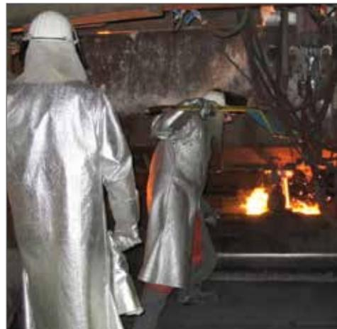
Fig. 2. Continuous casting of AMLoCor.
