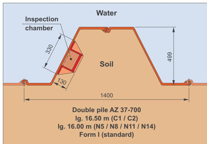
Fig. 9. Detail of a special sheet pile for monitoring the residual thickness.
