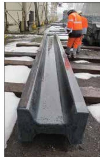
Fig. 8. AMLoCor beam blank used for rolling sheet piles.
