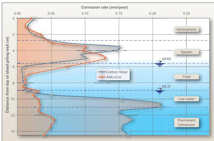
Fig. 1. Corrosion rates measured in a Northern European port.
