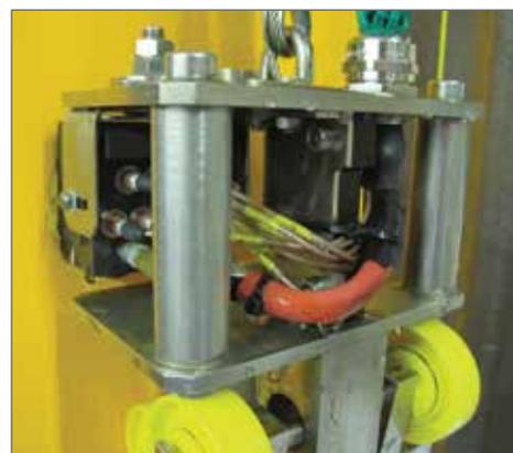
Fig. 7. Prototype of an ultrasonic measuring device.
