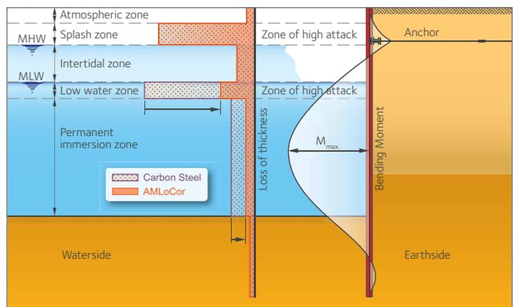
Fig. 4. Typical loss of steel thickness in a marine environment (MHW: Mean High Water; MLW: Mean Low Water).
