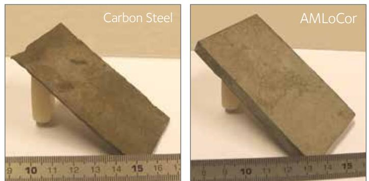
Fig. 3. 15 years old samples exposed in the water of a Northern European port.
