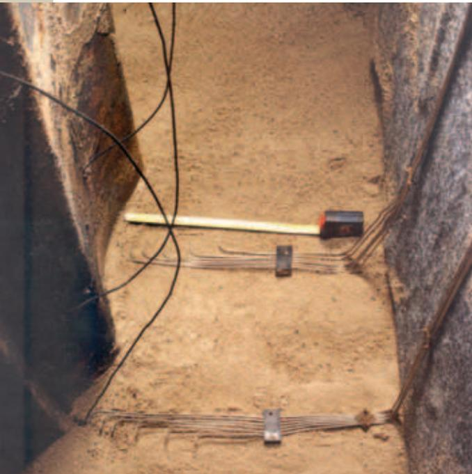
(Fig.29) Temperature gauges in the soil body
